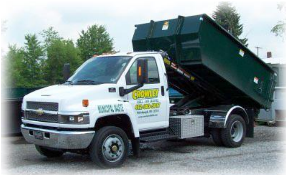
Crowley's truck outfitted with the Switch-N-Go system.
