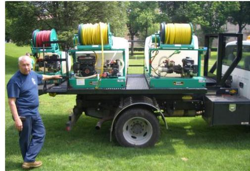
Sprayer units mounted to a Switch-N-Go subframe help the crew keep up with grounds maintenance.
